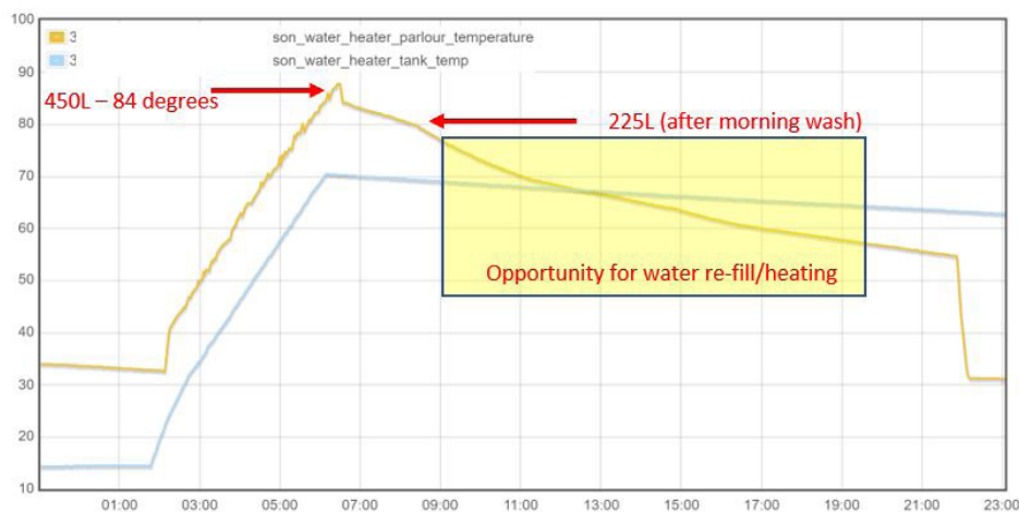
Figure 4.1 Hot Water Temperature: Parlour & Tank
