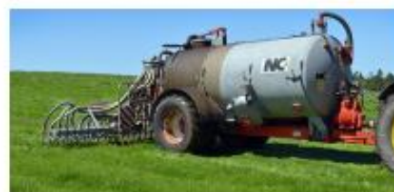
Trailing shoe reduces N loss and can improve yields by up to 25%
