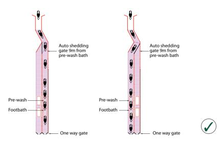
Fig 25 A double arrangement whereby a group of cows can be switched to a clean footbath
