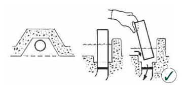
Fig 22 An alternative drainage arrangement for footbaths
